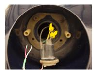
Plug the brake light LEDs into the brake light socket. Secure the brake light housing to the body but do not completely tighten the screws until the entire system is checked for proper operation.
