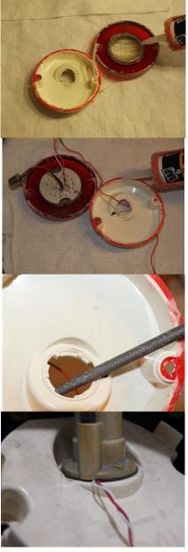
When reassembling the lens and housing, place a small bead of silicon around the outer edge of the lens. Ensure you do not fill the small hole in the housing or the area around the screw holes. The small hole allows air to flow in and out of the housing allowing heat to flow. Although
